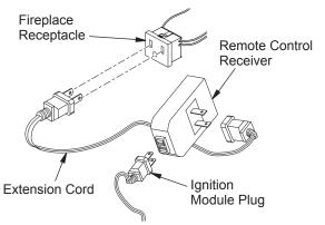
Figure 47 - Installing the WRC Remote Receiver
